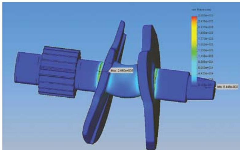
FEA diagram of the weld-up stock crankshaft depicting the predicted failure point of the crankshafts. This is exactly where the crankshafts failed in the actual race engines
