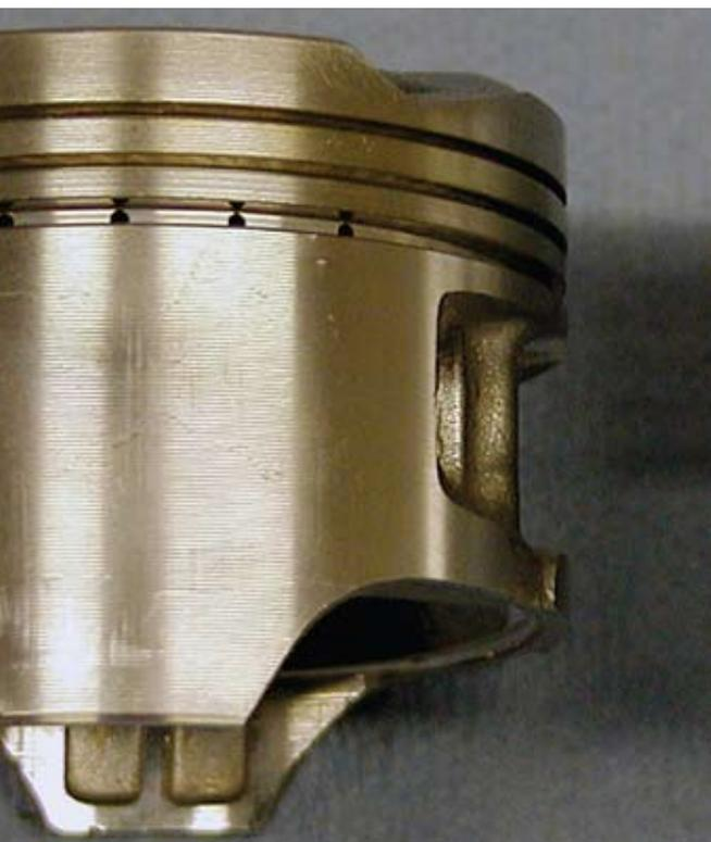
0.8mm (0.03") thick top and secondary compression rings as well as a 1.5mm (0.06") spring/twin-rail oil control pack. The wrist pins are full length steel pins with an outside diameter of 14.0mm (0.6"). Tying the pistons to the crankshaft are production-grade steel connecting rods, 100.0mm (3.9") from centre to centre, with rod bolt and nut fastening.
