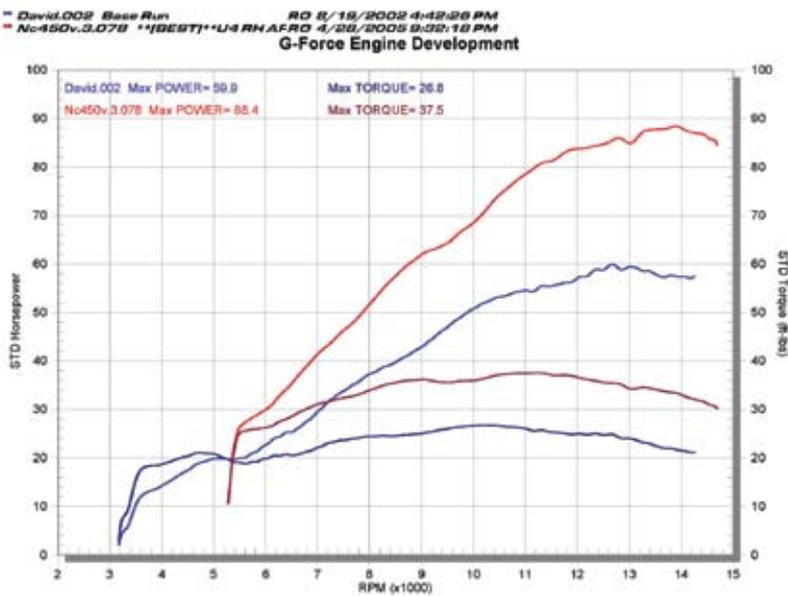
This graph shows the comparison of a stock motor (blue) and our 450cc motor as April 2005
