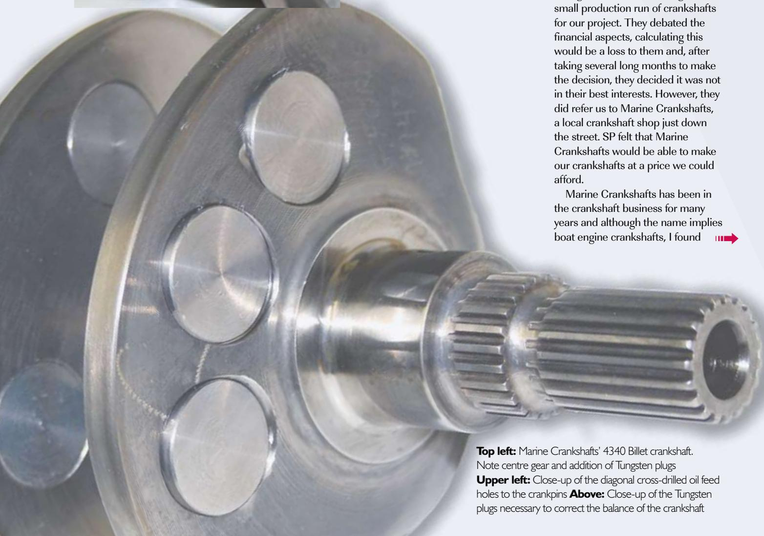
**Top left:** Marine Crankshafts' 4340 Billet crankshaft. Note centre gear and addition of Tungsten plugs
